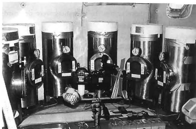
Fig. 1. Combustion chambers in NASA KC-135 aircraft laboratory
