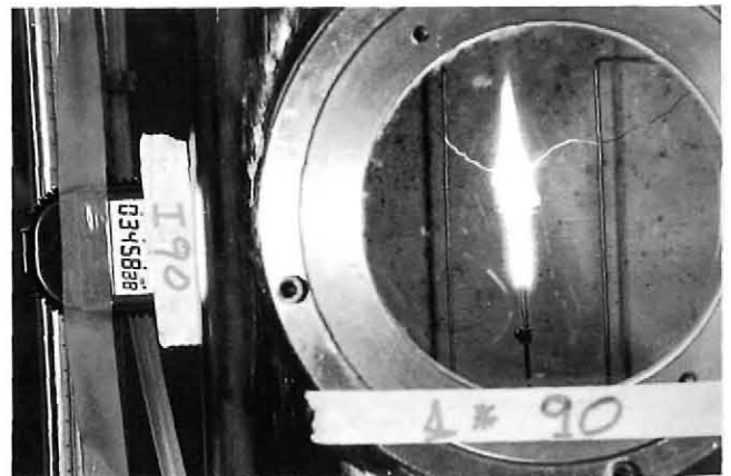
Fig. 10. Downward flame spreading over cylindrical samples at 1-g Y_{O_2} = 0.90 , P = 98 kPa
