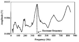
Fig. 1. Vibration response spectrum of a peach measured using a microphone
