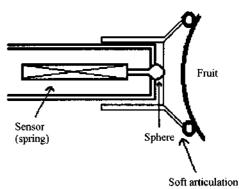
Fig. 2. Microdeformation based firmness sensor
