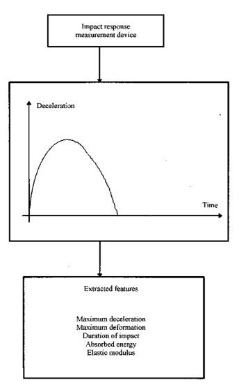
Fig. 3. Impact based firmness sensor
