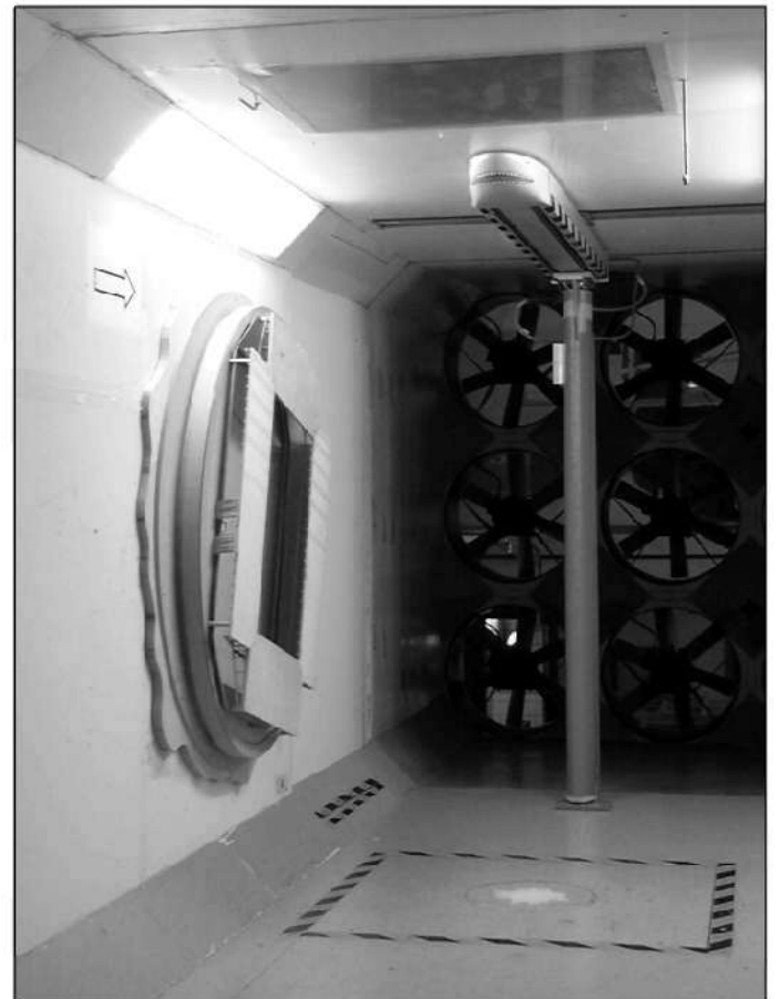
Figure 10. Testing model of the R.C.D. Espanyol football team's new stadium placed at the testing chamber of the A9 wind tunnel.
