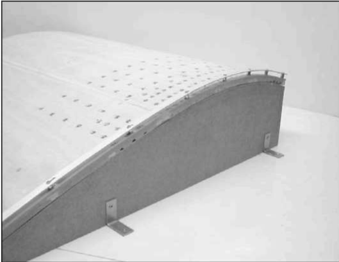
Figure 5. Cantilever parapet positioned on one of the eaves of a wind tunnel model's roof. The purpose of this research was to study the wind load on a curved roof and the effect of a cantilever parapet in order to alleviate it. See also Figure 6.
