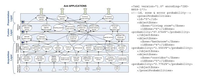
Figure 2. a) Service composition. b) Example of the ZigBee location service XML interface. It is the response to the HTML query http://server\_ip:8180/locationZigbee/proximityProb?id=5.
