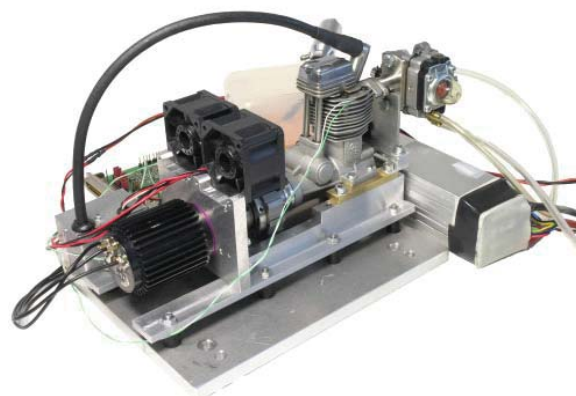
Figure 7. The individual parts of the realized prototype of Wearable Power System with total competition weight of 3989.6 grams. The system housing is not shown.
