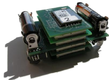
Fig. 2. Modular platform for wireless sensor networks, modeled and simulated in the present work.
