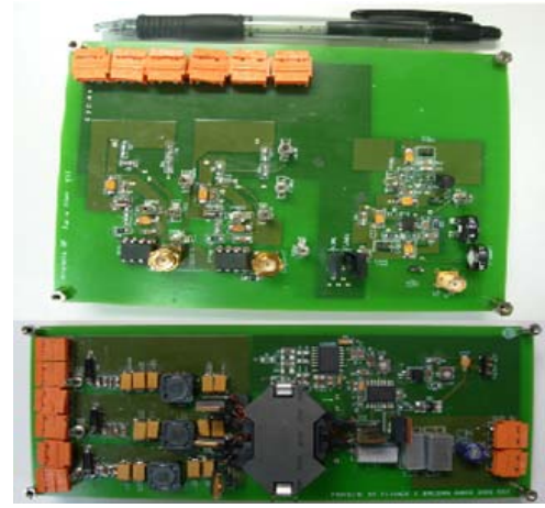
Fig. 13. Photograph of implemented multilevel converter, architecture two
