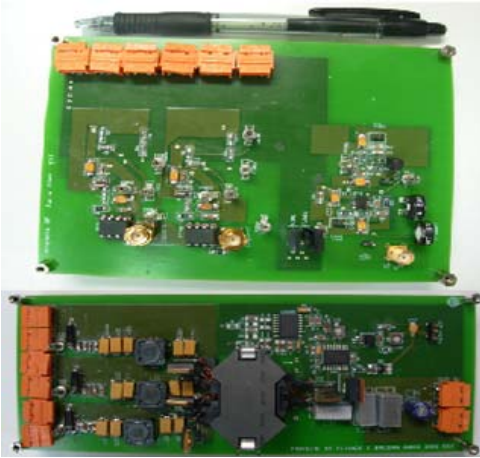
Figure 13. Photograph of implemented multilevel converter
