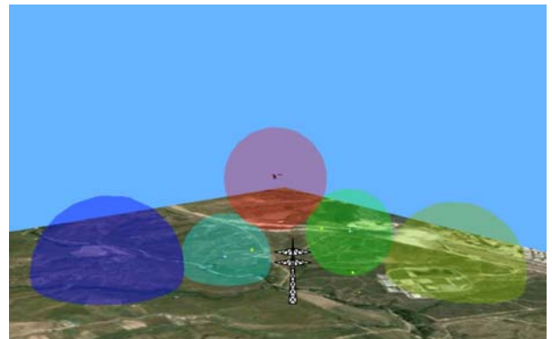
Fig. 6. Communication relays. Three aerial vehicles have to negotiate how to position themselves in order to guarantee communications between two fixed rovers' positions (leftmost and rightmost spheres). Spheres represent signal range. Note the presence of an obstacle in the middle (power tower).
