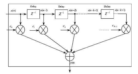
Fig. 2. An N-tap digital FIR filter.
