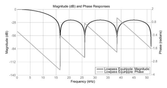
Fig. 3. Magnitude and the phase response of the FIR filter.
