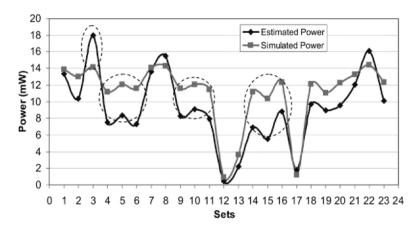
Fig. 4. Power comparison between macro-model and reference simulated power, Larger error spots for metric values between [0, 0.2] or [0.8, 1].
