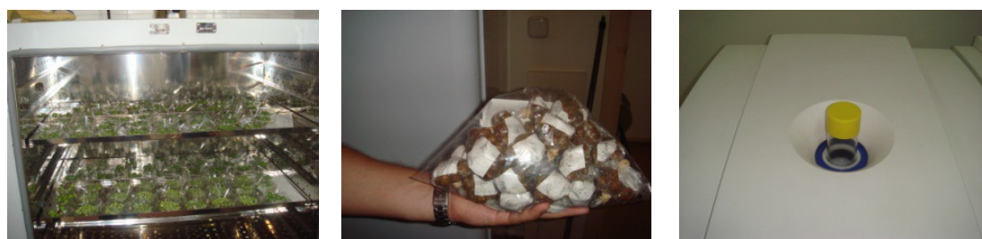
Figure 1 – Olive fruis dehydration in an oven (left), sample preparation in bags containing 10 fruits (middle) and Bruker Minispec equipment at IFAPA for low resolution oil content measurement.
