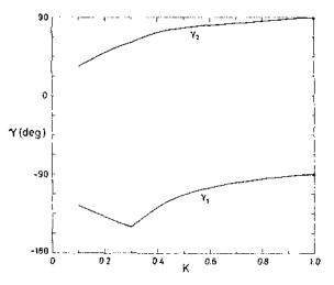
Fig. 6. Values of the minimum values of the angles at the smaller disk ( $\beta_1 = \gamma_1$ ) and the larger disk ( $\beta_2 = \gamma_2$ ) for critical bridges corresponding to the upper boundary and small values of the slender-tiess
