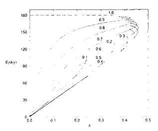
Fig. 16. Values of the angle at the smaller disk,  $\beta_1$ , for the limiting nodoid surfaces. Numbers on the curves indicate the disk radii ratio, K
