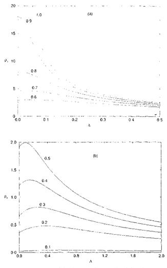
Fig. 8. Dependences of the dimensionless smaller disk radius,  $\varrho_1$ , on the slenderness, A, along the upper boundary of stability region. Numbers on the curves indicate the disk radii ratio, K
