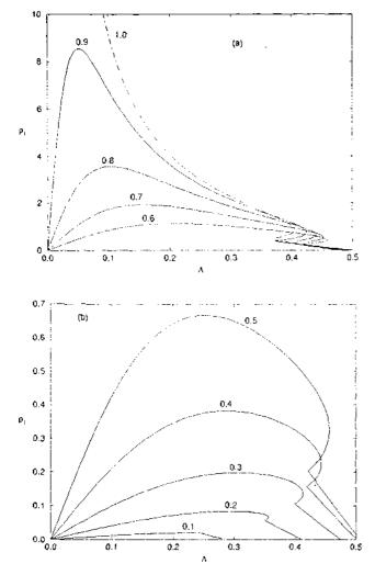
Fig. 15. Values of the dimensionless smaller disk radius,  $\varrho_1$ , depending on the slenderness. A, for the critical and limiting nodoid surfaces. Numbers on the curves indicate the disk radii ratio, K
