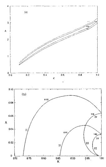
Fig. 18. Critical values of the slenderness, A, depending on disk radii ratio, K. Numbers on the curves indicate the relative volume, V
