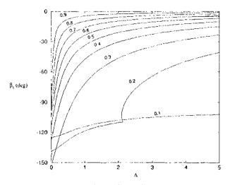
Fig. 4. Dependence of the angle at the smaller disk,  $\beta_1$ , on the slenderness, A, for critical bridges corresponding to the upper boundary of stability region. Numbers on the curves indicate the disk radii ratio, K
