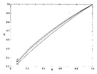
Fig. 20. Limit of minimum relative volume, V, depending on the disk radii ratio, K, for stable bridges with given values of the angle  $\beta_1$  on the smaller disk. Numbers on curves indicate the values of  $\beta_1$
