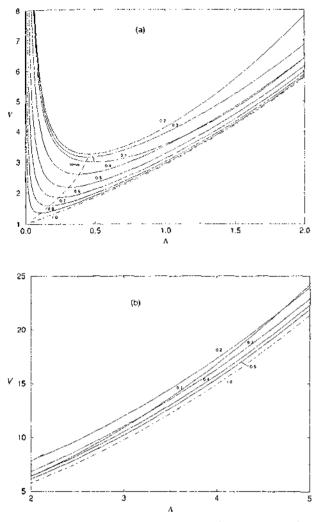
Fig. 9. Upper boundaries of stability region for small and middle (a) and large (b) values of the slenderness, A, and different values of disk radii ratio, K. Numbers on the curves indicate the values of K. The dotted line in (a) joins the points of minimum V for given K.
