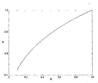
Fig. 17. Dependence of the relative liquid volume,  $V = V_0$ , for small values of slenderness on the disk radii ratio, K, for the limiting nodoid surfaces
