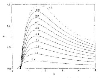
Fig. 14. Values of the dimensionless smaller disk radius,  $q_1$ , depending on the slenderness,  $A_s$  for the critical unduloidal surfaces. Number on the curves indicate the disk radii ratio, K
