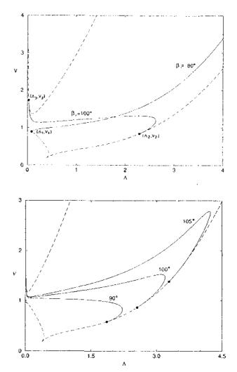
Fig. 19. Boundaries of the stability region of liquid bridges with a disk radii ratio of (a) K = 0.8 and (b) K = 0.9 (dashed lines). The solid lines correspond to given values of (a)  $\beta_1 = 80$  and  $\beta_2 = 100$  and (b)  $\beta_1 = 90^\circ$ ,  $100^\circ$ ,  $105^\circ$
