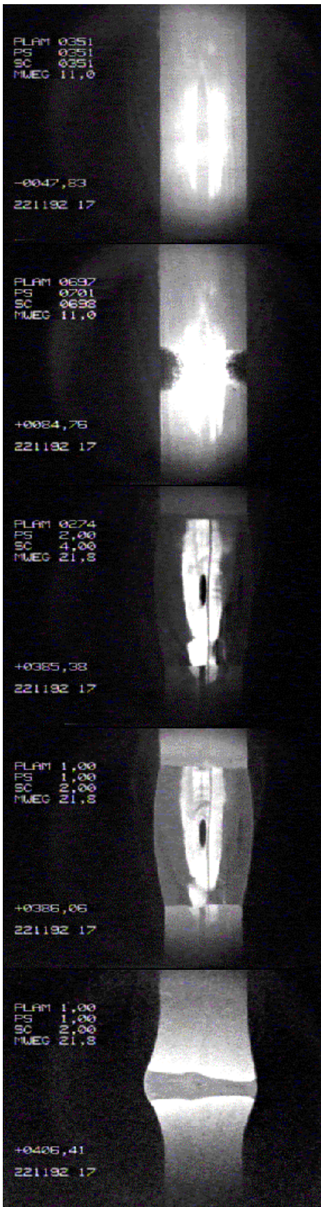
Fig. 3. Selected video-frames from a Texas experiment on floating-zone crystal growth of silicon rod 8 mm in diameter inside a mirror furnace [Ref. 5], to give an idea of the difficulties in visualisation. The first one shows the silicon rod still being heated to melt; on the second one a short molten zone has formed; on the third one a long floating zone (more than twice its diameter) is (hardly) seen; on the fourth one the whole geometry is better seen just after switching off the furnace power
