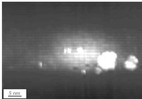
Figure 5.20 Topography image of an InAs/GaAs QD capped with InGaAs ( V = -3\text{V} , I_{\text{tunnel}} = 55\text{pA} ). The big white regions are cleavage induced defects. Growth direction: [001] , lateral direction: [110] .
