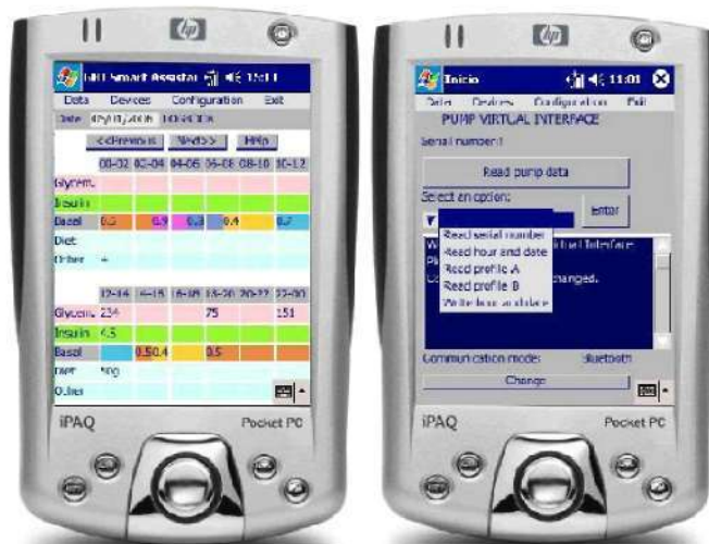
Fig. 2. The 'logbook' and pump communication scenarios for the PDA application and IPAQ h2210 PDA
