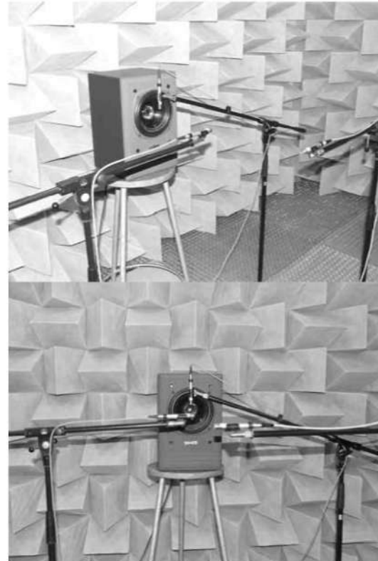
Figure 9 Loudspeaker and microphones disposition inside anechoic chamber
