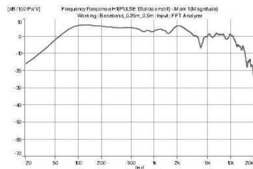
Figure 10 Loudspeaker frequency response as a transfer function between mic1 and power amplifier
