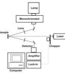
PR is a spectroscopy technique based on analysing the optical response of a material under a periodical light perturbation [Car69].
