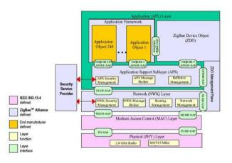
Fig. 3 ZigbeeTM stack protocol
