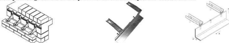
Figure 2. Standard European brackets anchored to a rail, embedded in the face of the slab.
