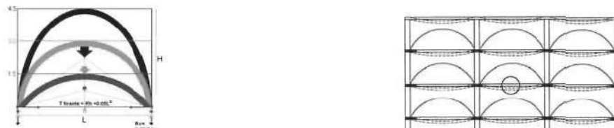
Figure 5 a) Braced arches of different heights all fitted with the same section of steel bracing; b) Braced masonry facing wall set on a framed structure and using the arch effect.
