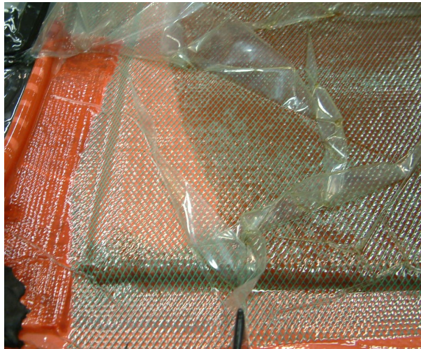
Fig.2. Vacuum infusion process for manufacturing of the hybrid laminate.
