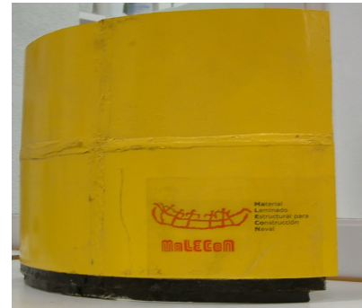
Fig.5. Assembly of curved panels
