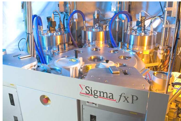
Figure 1. Sputtering tool used for the deposition of AlN films
