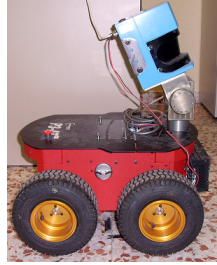
Fig. 1. Our robot Nemo equipped with a laser mounted on a wrist for 3D data acquisition
