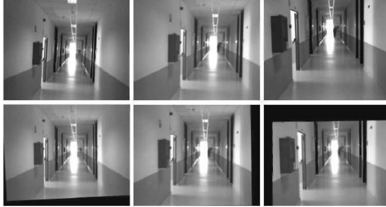
Fig. 6. A selection of frames (respectively 16, 88 and 120) of the sequence ‘corridor’ before (upper row) and after (bottom row) the video stabilization with N_w = 35
