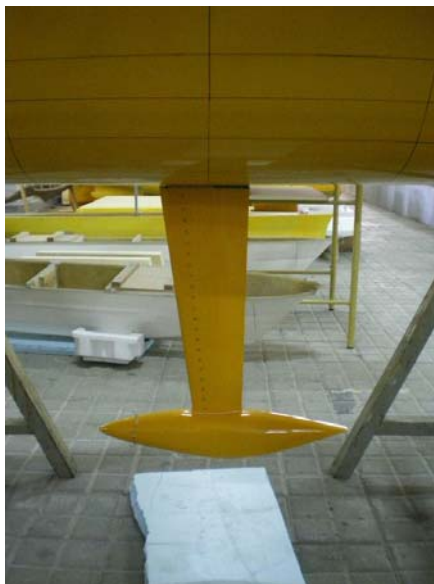
Figure 1: Turbulence Stimulators on hull, keel and bulb
