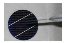
Figure 7 : Extremely thin (80  $\mu m)$  screenprinted solar cell with an efficiency of 16.6 %
