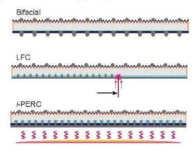
Figure 3: The passivated rear surface solar cells on low cost substrates can be classified in three groups: bifacial solar cells with fire-through contacts, laser fired contact solar cells, and selective alloying, thermally fired LBSF solar cells (i-PERCs)
