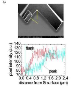
Figure 4: Emitter profile measured by secondary electron SEM. Darker regions correspond to n-type silicon. a) spray-on in-line diffusion, b) POCl<sub>3</sub> sample. The profiles are in both case about 0.5-1  $\mu$ m at the pyramid flank, and  $\sim$  1-1.5  $\mu$ m at the peaks.
