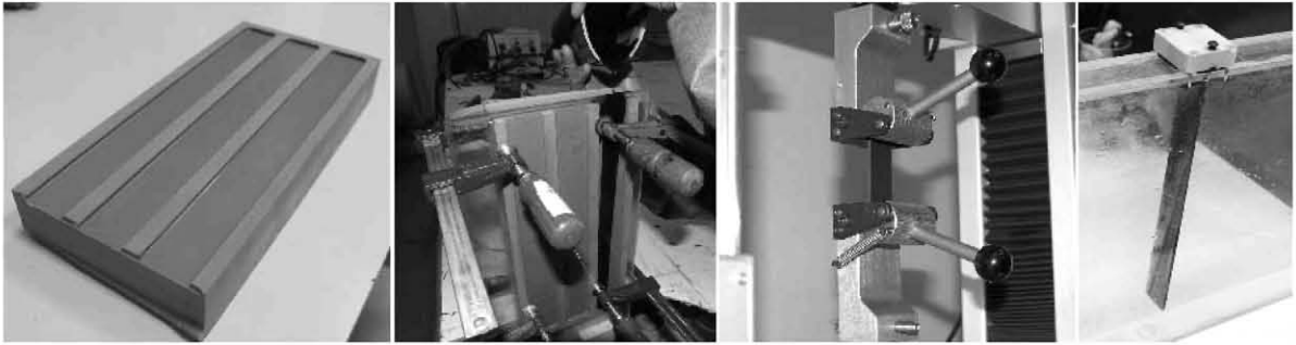
FIGURE 5: Mould for the probes, synthesizing process, traction test and anchorage
