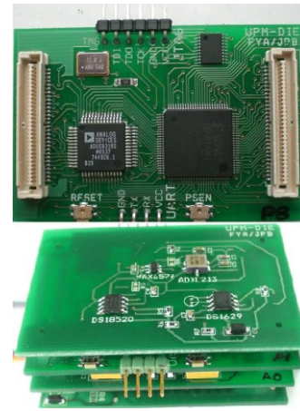
Fig. 1 Processing layer (uC on the left, FPGA on the right) and full Cookie platform
