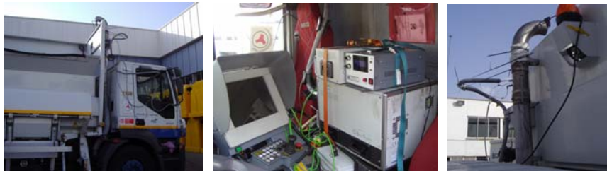
Fig. 3. Installation of the measurement equipment in a refuse truck with lateral loading.
