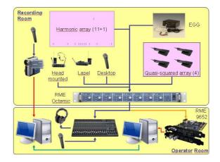
Figure 2: Schematic of recording setup
