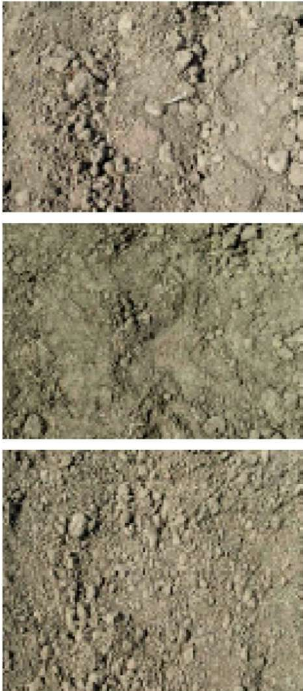
Fig. 5. Experimental sandy clay loam at the Spanish National Research Council's La Higuera site, after tilling with a chisel, top, roller (middle) and tiller (bottom).
