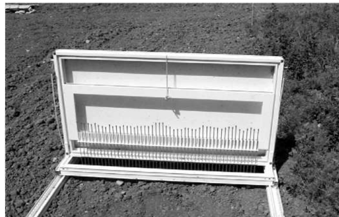
Fig. 7. Pin meter prototype, in the field.
