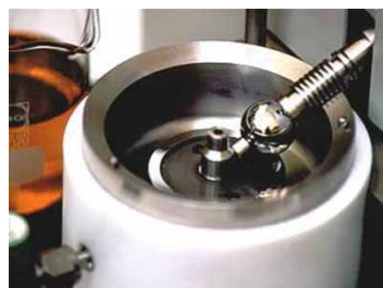
Fig. 2 Photograph and diagram of the test zone in the MTM
