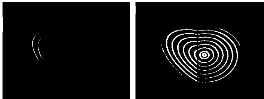
Fig. 15. View of surface discontinuity from laser-camera. Experiment 2.
