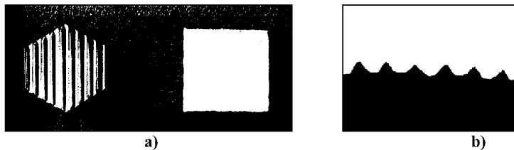
Figura 1. a) Cu and Al samples to be welded; b) cold welded joint on cogged surface
