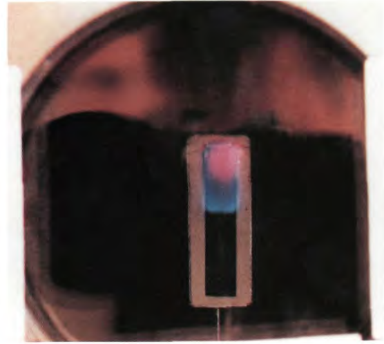
Figure 1.20 (cont.). Flame spreading over flat samples at microgravity conditions in the NASA KC-135 aircraft laboratory. Y_{O_2} = 0.80 , P = 50 \text{ kPa} .
