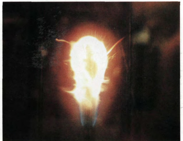
Fig. 1.15 Flame spreading over cylindrical samples at microgravity conditions in the NASA KC-135 aircraft laboratory. Y_{O_2} = 0.80 , P = 20 kPa.
