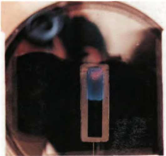
Figure 1.20 (cont.). Flame spreading over flat samples at microgravity conditions in the NASA KC-135 aircraft laboratory. Y_{O_2} = 0.80 , P = 50 \text{ kPa} .
