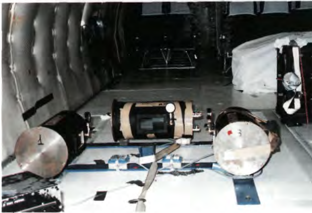
Figure 1.1. Combustion chambers in the NASA KC-135 aircraft laboratory. First campaign.
