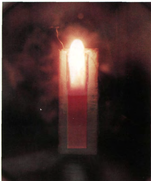
Figure 1.9. Downward flame spreading over flat samples at 1 g. Y_{O_2} = 0.90 , P = 98 kPa.
