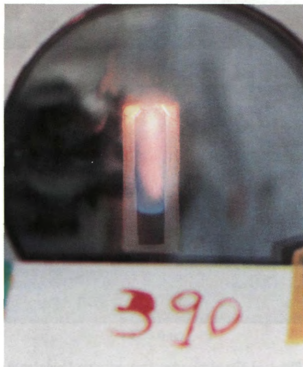
Figure 1.10. Downward flame spreading over flat samples at 1 g. Y_{O_2} = 0.90 , P = 30 kPa.
