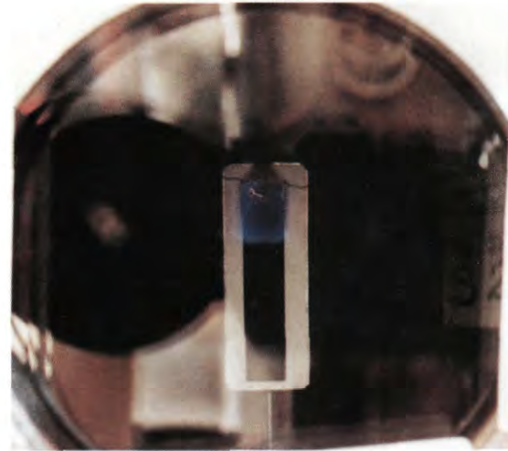
Figure 1.21. Flame spreading over flat samples at microgravity conditions and different O_2 mass fractions. NASA KC-135 aircraft laboratory.
