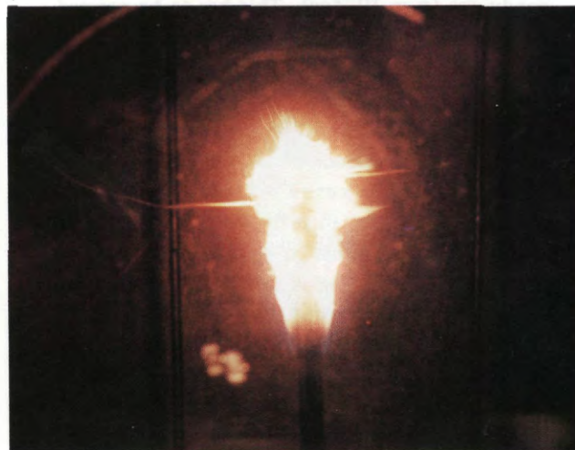
Fig. 1.14 Flame spreading over cylindrical samples at microgravity conditions in the NASA KC-135 aircraft laboratory. Y_{O_2} = 0.90 , P = 50 kPa.
