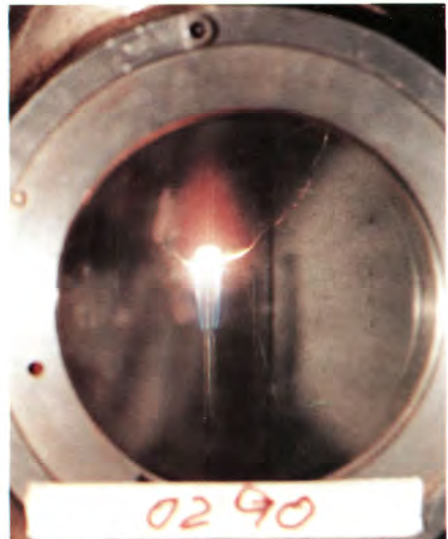
Figure 1.8. Downward flame spreading over cylindrical samples at 1 g. Y_{O_2} = 0.9 , P = 20 kPa.
