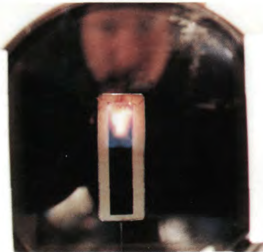
Figure 1.21. Flame spreading over flat samples at microgravity conditions and different O_2 mass fractions. NASA KC-135 aircraft laboratory.
