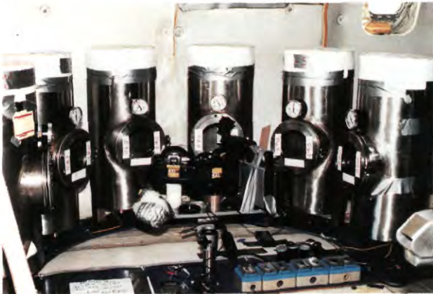
Figure 1.2. Combustion chambers in the NASA KC-135 aircraft laboratory. Second and third campaigns.
