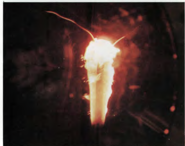
Fig. 1.13 Flame spreading over cylindrical samples at microgravity conditions in the NASA KC-135 aircraft laboratory. Y_{O_2} = 0.90 , P = 98 kPa.
