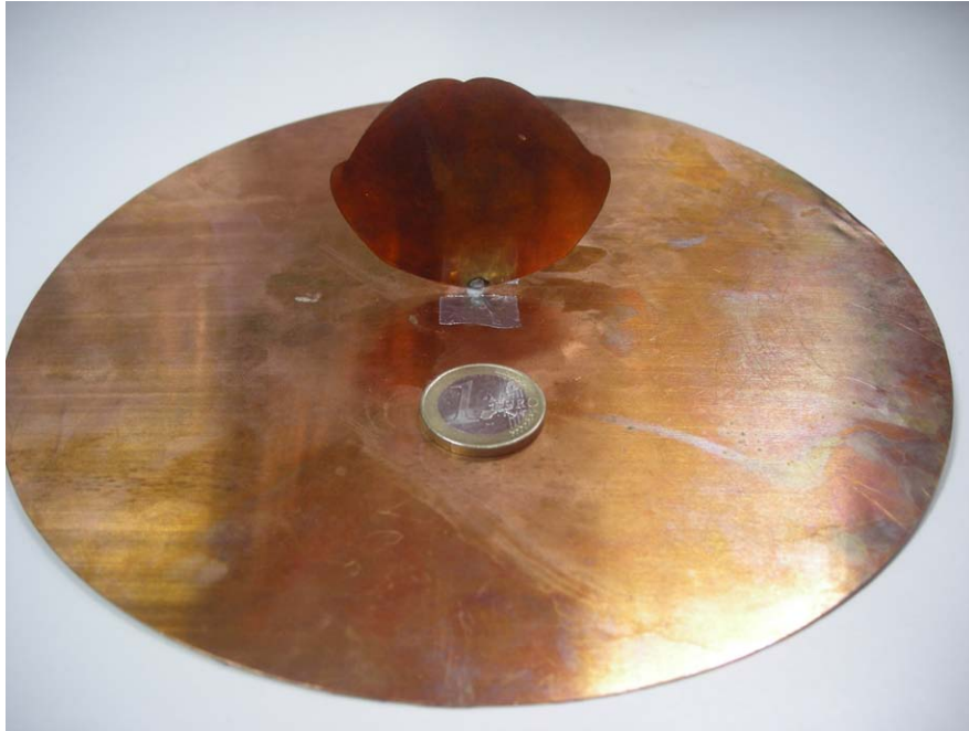
Figure 10.38: Pure global optimization method antenna prototype photograph compared with an euro coin
