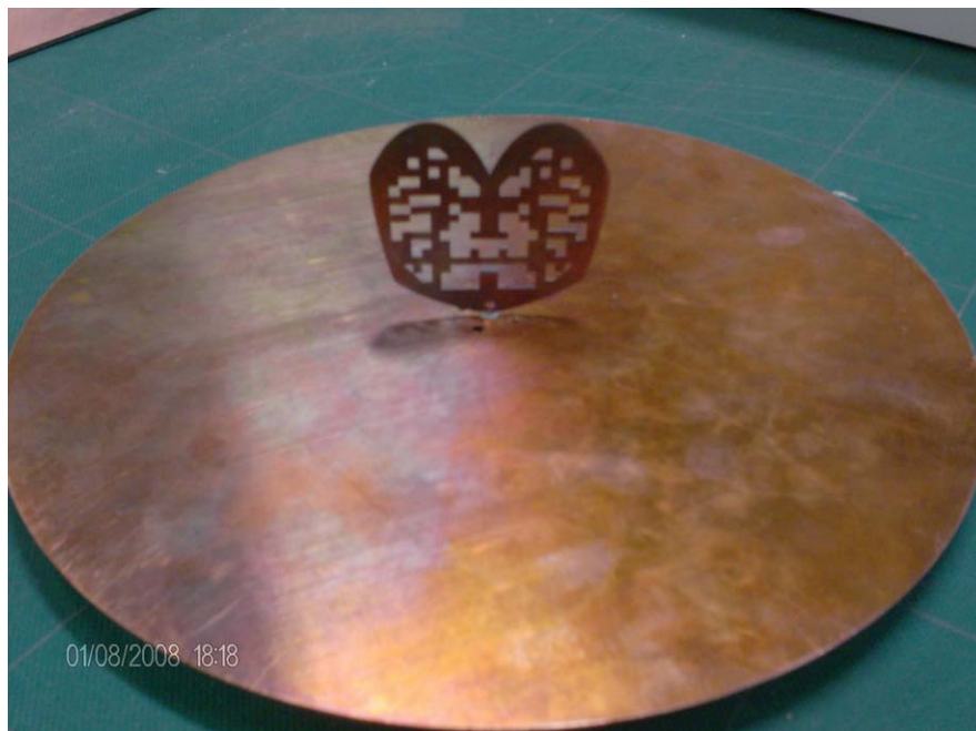
Figure 11.3: Photograph of the built prototype with the first cost function, including 10cm. radius ground plane
