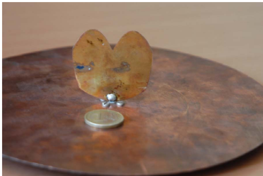
Figure 10.18: Hybrid method antenna prototype photograph compared with a euro coin
