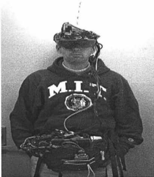
Figure 1.2(a) Smart clothing. Smart wearable devices worn include the wearable multimedia computer/personal visual assistant. The eyeglasses include a miniature computer screen and sensor array. The equipment also supports an Internet connection (Mann, 1996)
