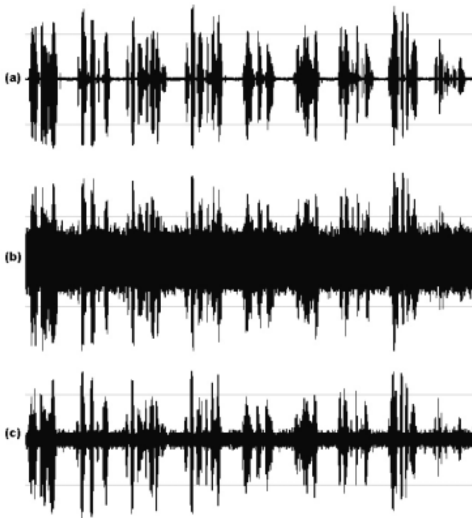
Fig. 5. Original signal (a) plus noise (b) and smoothed estimate (c)
