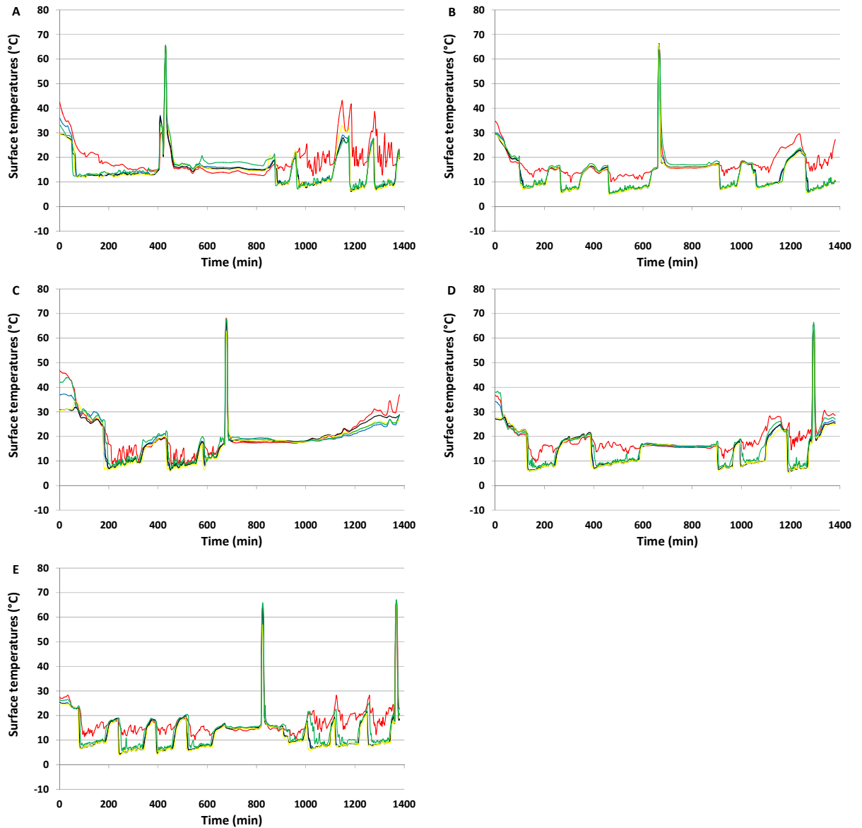
Figure 3.a-4 In total, five different milk tankers were monitored during summer of 2010. Each graph represents the surface temperature of a milk tanker over a period of 23 h.
