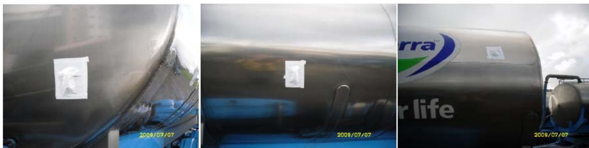
Figure 3.a-3 The affixation of the data loggers on the outer surface of a milk tanker.
