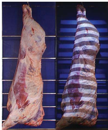
Figure 2.1 Two-dimensional (left) and pseudo three-dimensional (right) images from the VBS 2000 (Image courtesy of E+V GmbH, Germany).
