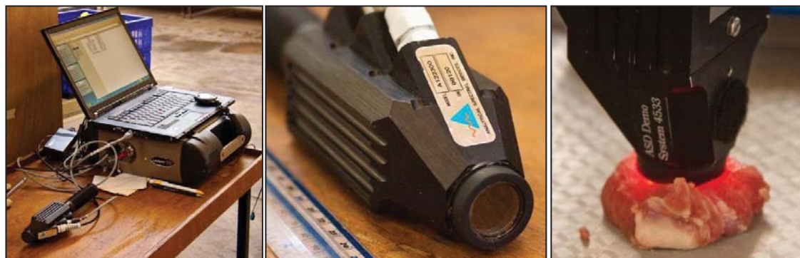
Figure 6.1 The ASD Labspec 5000 NIR spectrometer (left), the high intensity contact probe (centre) and application to a slice of lamb LL (right).
