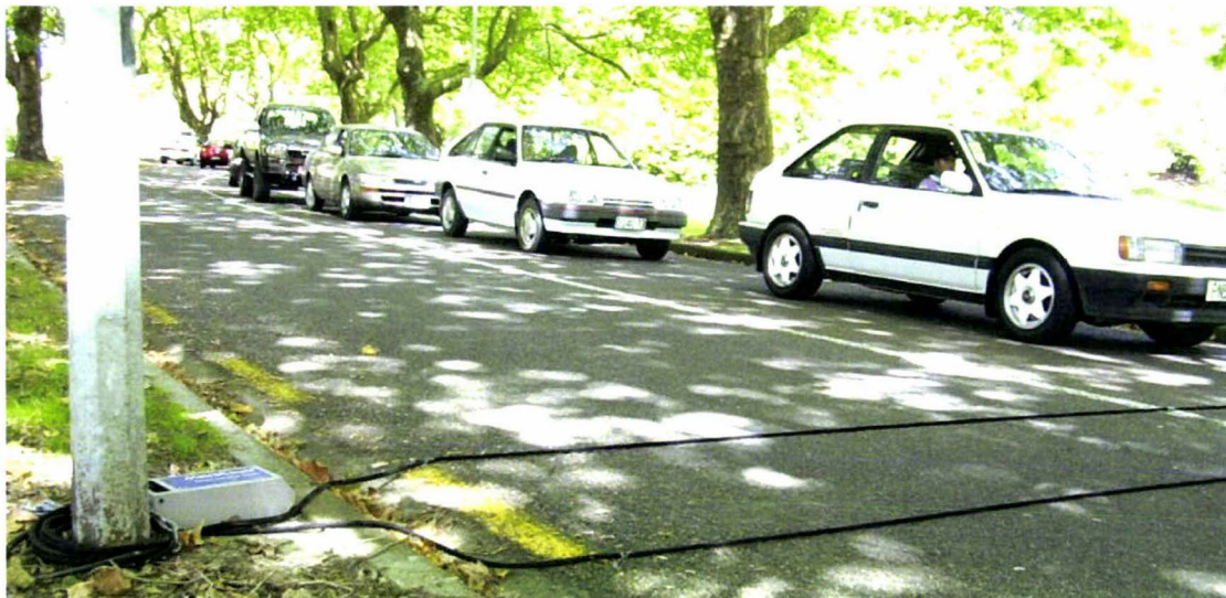
Figure 3.3: MetroCount vehicle counter installed at the Massey main entrance
