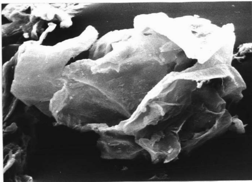
Figure 3.12: Wall prepared by wet sieving (Batch 1). Scanning E.M. 1400x
