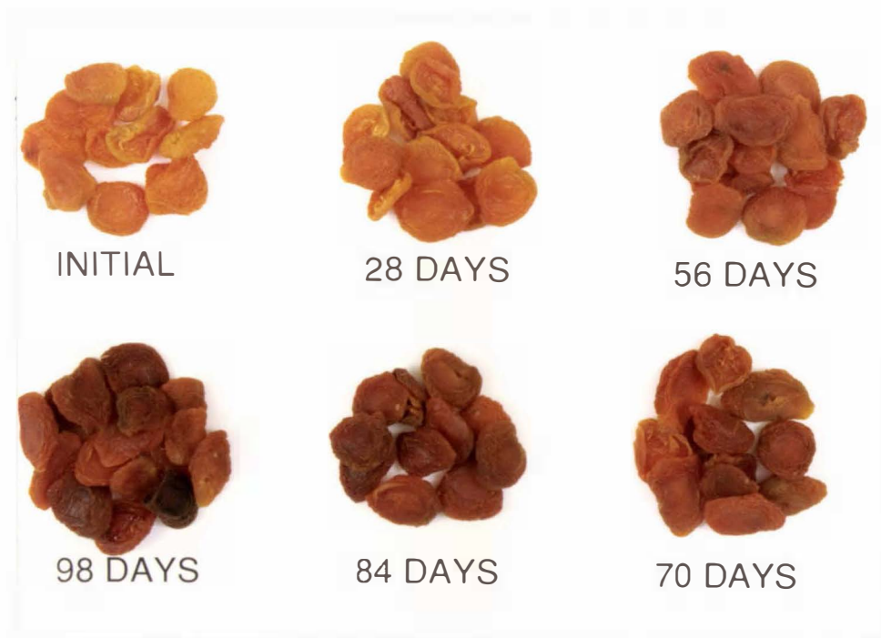
Fig. 4.31 . Change in colour of dried apricot halves, packaged in LDPE film, during storage at 30°C/75%RH.
