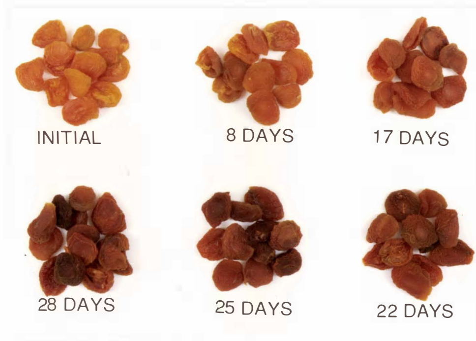
Fig. 4.32 . Change in colour of dried apricot halves, packaged in LDPE film, during storage at 40°C/90%RH.
