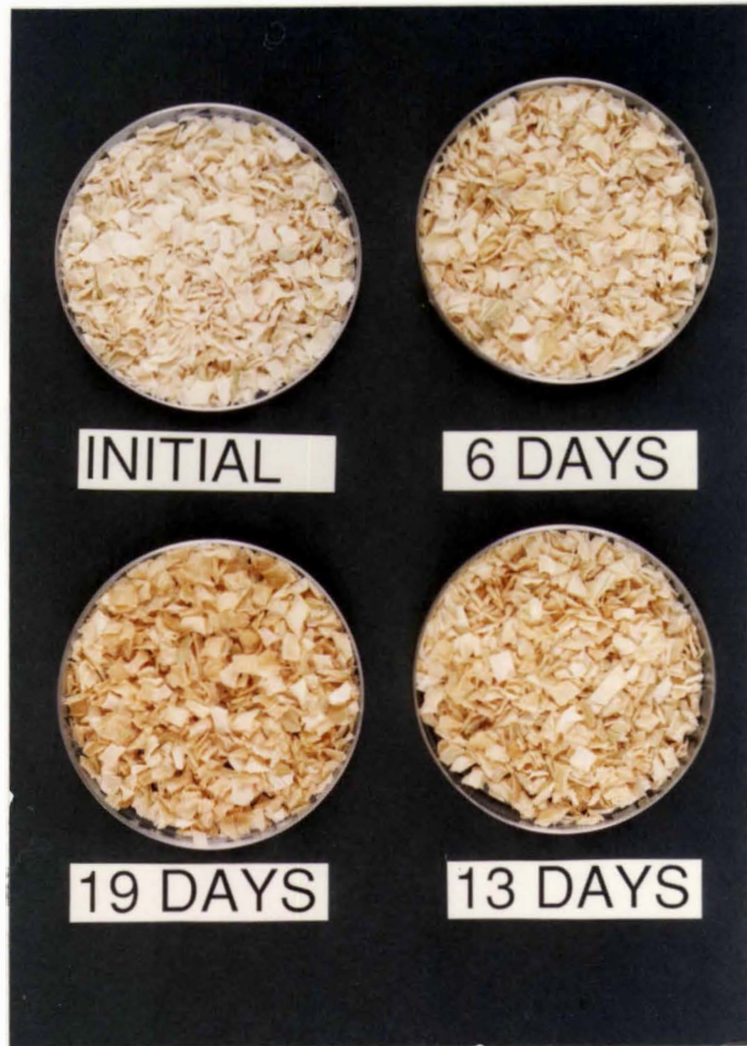
Fig. 4.5. Change in colour of dried onion flakes, packaged in LDPE film, during storage at 40°C/90%RH.
