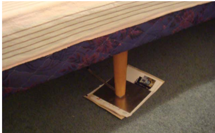
Figure: 4.10: The placement of a sensor under a leg
