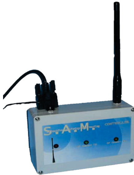
Figure 3.27: Picture of the fabricated unit of the Central Control Unit
