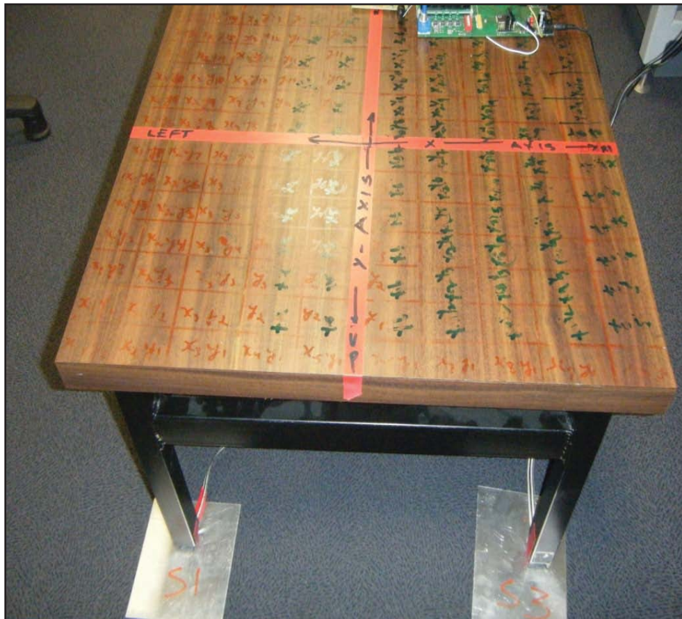
Figure 3.11: Experimental Setup with four force sensors
