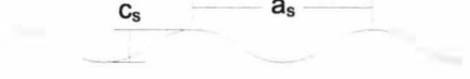
Figure 2.4: Sinusoidal Sample Model: Chen [44] as well as Binnig and Rohrer [27] assume this sample surface to estimate the lateral resolution of the s -wave tip model of Tersoff and Hamann [181].
