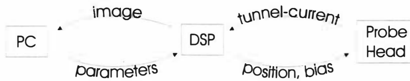
Figure 1.3: Interaction between PC, DSP and Probe Head: The DSP assumes a central position between PC and probe head. Not only does the DSP control the the tip-sample distance, but it also exchanges image and control data with the PC. The interaction labels indicate the main purpose of the link. Note that the DSP also controls the horizontal position and the coarse movement of the probe head.
