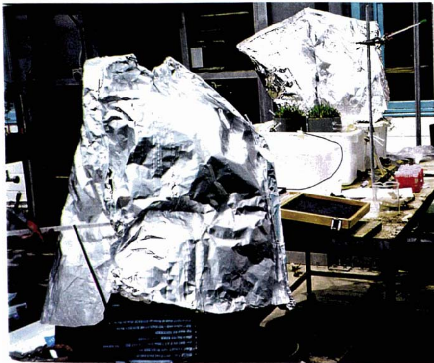
Plate 7.3: Monitoring temperature fluctuations inside of the dark canopy placed over another soil core (i.e. not used for pulse labelling study) in the open environment.
