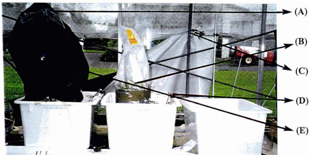
Plate 7.1: The ^{14}\text{CO}_2 pulse labelling system. Dark (A) and light (B) lysimeters placed in sand baths (on the left hand side) and connected to a water bath (on the right hand side). Also showing (C) thermometer for noting glasshouse temperature, (D) quantum sensor for PAR measurements, and (E) 3-way stopcock on the dark bag for sampling and injecting ^{14}\text{CO}_2 .
