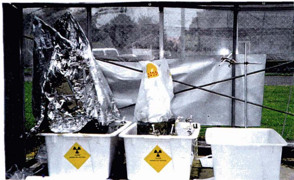
Plate 7.2: The ^{14}\text{CO}_2 pulse labelling system, after injection of ^{14}\text{CO}_2 pulse. Aluminium foil cover is in place over the dark polyethylene bags on 'dark' soil cores to control temperature rise inside the bag.
