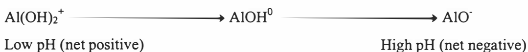
Figure 2.1 Development of variable surface positive charge through the dissociation or association of \text{H}^+ on a mineral surface (Bolan et al. , 1999).
