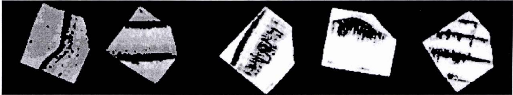
300 MHz ^1\text{H} magnetic resonance image of wood samples in transverse section
