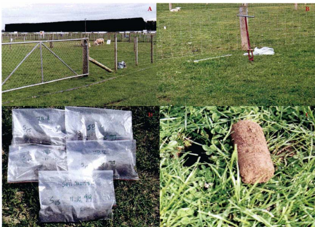
Figure 2-1 Soil sampling process
