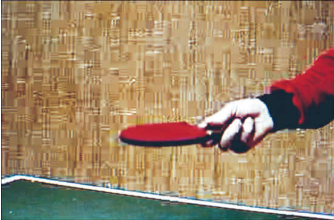
Figure 4.17 From Yuen and Wu [27] illustrate colour ringing and colour blurring of the chrominance: “the reproduction of a frame suffering from colour bleeding and colour ringing from the Table-tennis sequence. Note the high-frequency changes in colour around the table edge, corresponding to the ringing, and the gradual bleeding around the arm”.
