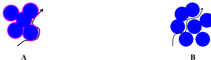
Figure 5-3 Conceptualisation of diffusional modes within the bed (given negligible concentration gradient within particles): Particle surface diffusion, where the magenta rings represent thin films through which diffusion occur (A), and gas phase diffusion within voids available between particle (B).
